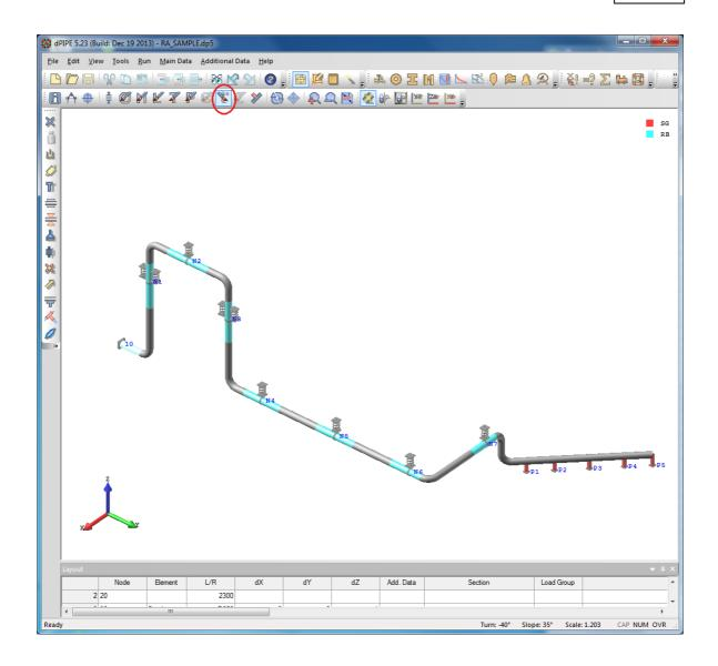
13. Specify the method of analysis for dynamic analysis (<u>DYN</u>) as the response spectrum method (RSM), limit frequency <u>FMAX</u> as 33 Hz and the parameter for automatic breakdown of the model <u>FMESH</u> as 60 Hz ("Service\Options\Reference parameters\Dynamic" menu):
