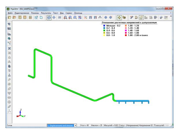
View the results on the selection of springs of spring hangers/supports ("Loads on supports", button) :
