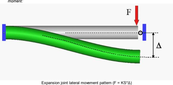
corresponds to the deformation of a cantilevered beam under the action of concentrated moment:
