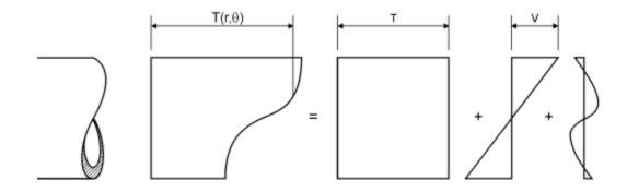
Decomposition of Stratification Temperature Distribution Range.
