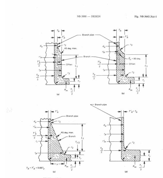
GENERAL NOTE: If  $L_1$  equals or exceeds 0.5  $\sqrt{r_i T_b}$ , then  $r'_m$  can be taken as the radius to the center of  $T_b$ .
