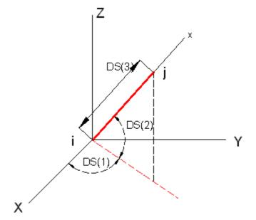
Determination of the element direction in the spherical coordinate system
