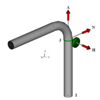
Direction of local coordinates of the support for a vertical piping segment
