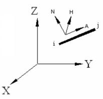
3. If the local A axis is parallel to the global Z axis, then the local H axis coincided with the global Y axis, and the local N axis is constructed according to the right-hand rule (N = A x H)
