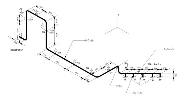
Figure 1. Isometric diagram of the sample piping system
