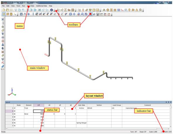
The *main window* of the program displays either the graphic model the piping system, or the model description in the form of a set of commands of the dPIPE software <u>input data entry language</u>.
