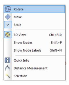
Rotate ( ): rotation of the model by means of the mouse with the left button being pressed;
