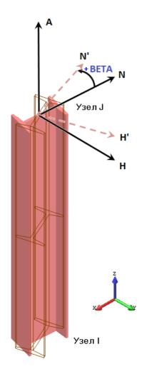
2) the local A axis is parallel to the global Z axis (H is directed along the global Y axis).
