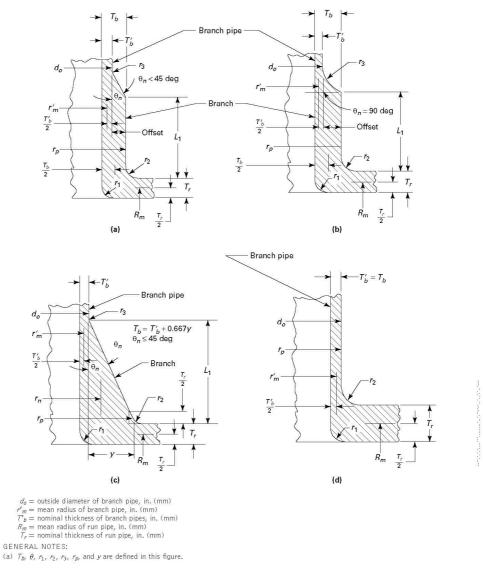
FIG. NC-3673.2(b)-2 BRANCH CONNECTION NOMENCLATURE
