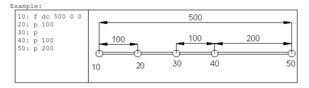
In this example the length of element 20 - 30 is automatically computed as 500 - (100 + 100 + 200) = 100
