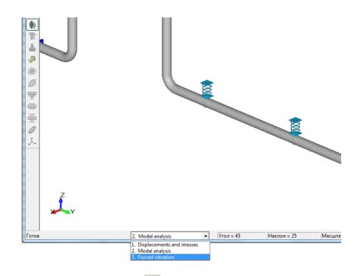
and then it is possible to use *and* and *buttons for viewing the animation.* It should be kept in mind that when the forced vibration is recorded the size of the <model>.bin file will increase significantly!
