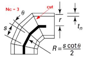
If Nc = 1 the radius (R) should not be set: the program will determine it based on the relation:  $Re = 0.5 * r * (1 + ctg (\theta))$ , where: r is the mean radius of the pipe;  $\theta$  is half the total angle of the bend. If Nc > 1, then  $\theta = \alpha/(2*N_c)$ , and  $s = 2*R_e*tg(\theta)$
