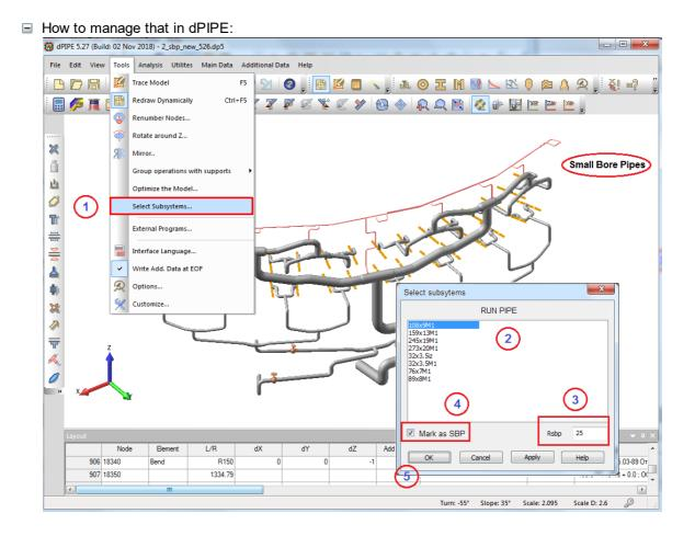
2. Run conventional seismic analysis of the whole system. Resulting internal forces in the small bore pipes would consist from the combination of the primary (inertial) seismic loads,  $F_{SBP}^{INRT}$ , and secondary (displacement based) components,  $F_{SBP}^{SAM}$ :
