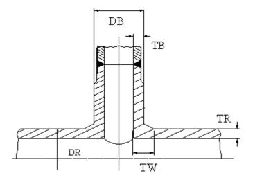
Cross-section of the tee joint (Russian PNAE Code)
